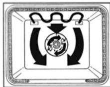
The top element operates at full power whenever heating. It will cycle on and off to maintain the set temperature. Air in the oven cavity is circulated by the fan for even heating. Use this setting for broiling thicker cuts of meat, poultry and fish.
