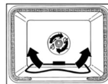
The bottom element operates at full power whenever heating. Air in the oven cavity is pulled into the center of the fan and pushed out around the baffle for even heating and faster cooking.
